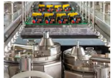
Innovative Y/Z-variable dual solder pot system
