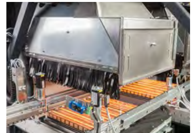
Speed regulated, full area convection for individual preheating performance
