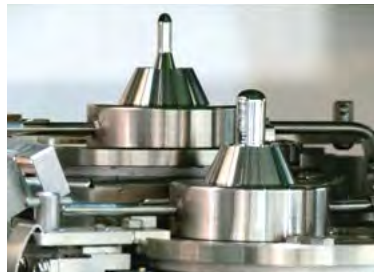
Dual solder pots with soldering nozzels in different shapes
